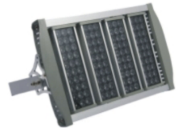
RG-MLW120-240W Lamp Power: 120X2W Working Voltage: 90-295V LED Color: □■□ Size: 536 X 310 X 70mm
